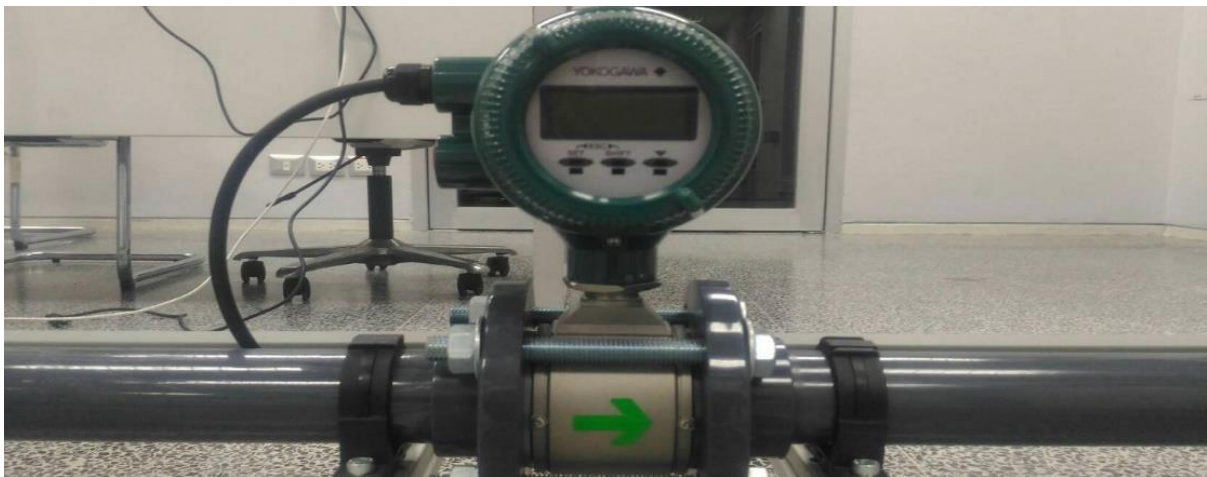
Fig. 5. The standard electromagnetic flowmeter.
