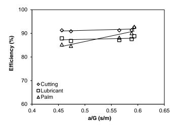
Fig. 3. Treatment efficiency versus a/G ratio for three oily-wastewaters at optimum coagulant dosages.
