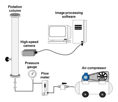
Fig. 1. Experimental set-up of induced air flotation process.
