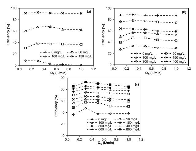
Fig. 2. Removal efficiencies with gas flow rates by MIAF of (a) cutting oil; (b) lubricant oil; and (c) palm oil.
