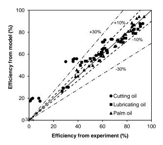
Fig. 4. Treatment efficiency of the constructed model compared to the experimental results.
