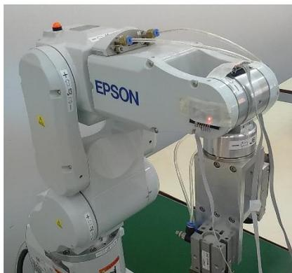
Fig. 7. Accelerometer on EPSON CA-A601S robot.
