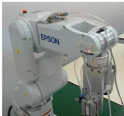
Fig. 7. Accelerometer on EPSON CA-A601S robot.
