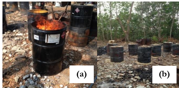
Fig. 3. (a) Fire was dispersed among all the 200-L tanks; (b) Raw materials were carbonized in the closed 200-L tanks for 24 h.
