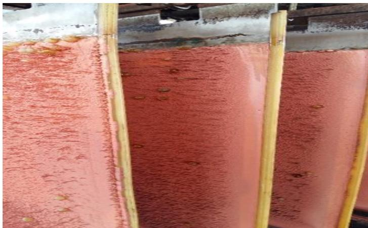
Fig. 13. Physical aspect of cathodic copper when solid colloidal particles and silica are present in aqueous solution at copper solvent extraction
