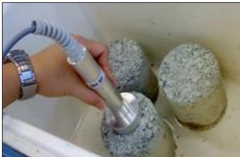
Fig. 5. Measurement of Dielectric Value, DV.
