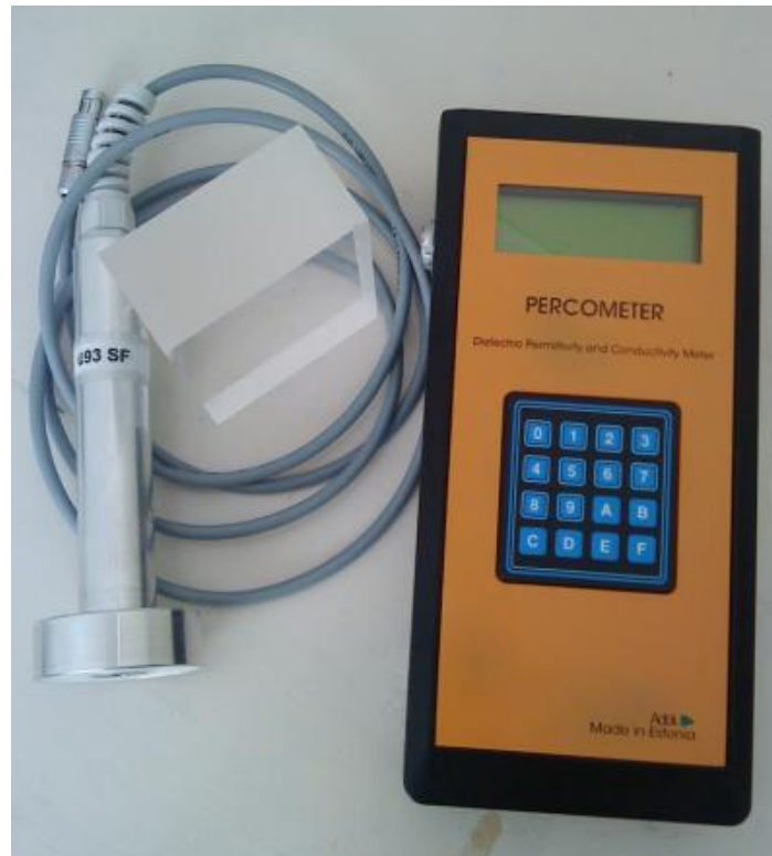
Fig. 3. Percometer with Surface Probe.
