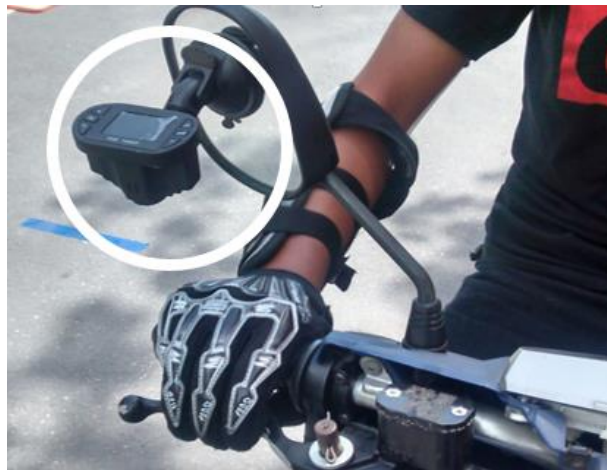
Fig. 4. Video recording device to monitor the number of finger actuation.
