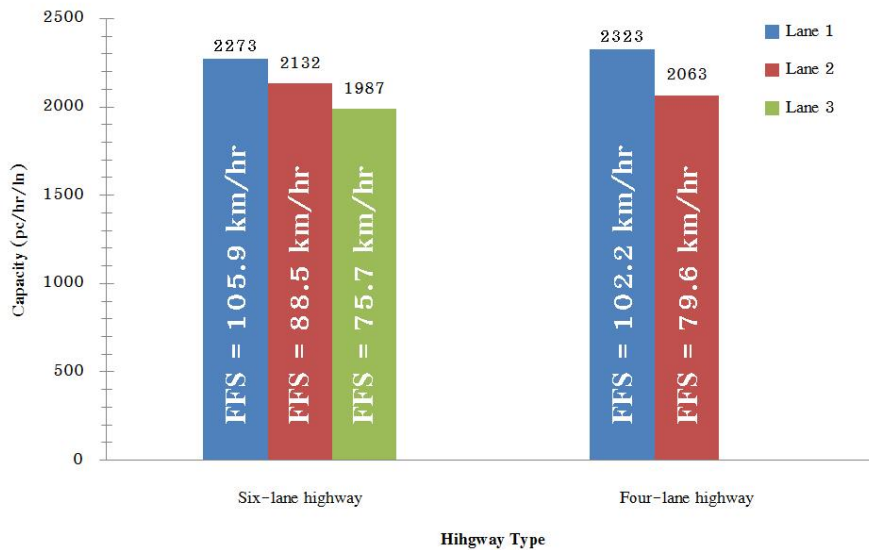
Fig. 7. Average capacity per lane for six-lane and four-lane primary highways.
