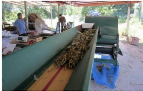
Fig. 2. The feed conveyor with adjustable feed rate.
