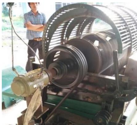
Fig. 1. Guide vanes attached to the upper concave drum.
