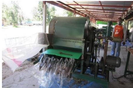
Fig. 3. Testing of soybean threshing unit at a workshop.
