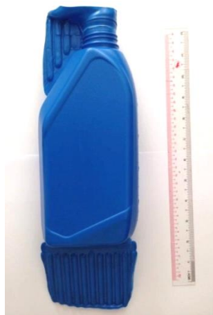
Fig. 2. The 1.0 liter lubricant oil bottle with flash or scrap.
