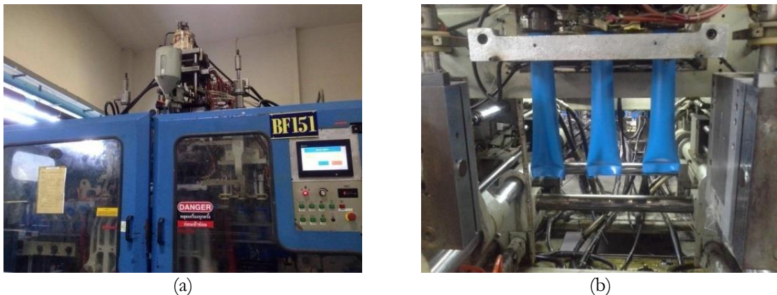
Fig. 1. (a) the extrusion blow molding machine, and (b) the parison extruding through the shaping dies of blow molding machine.
