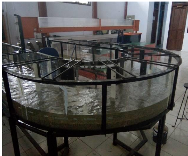
Fig. 2. Flume bend of 180°, width of 0.5 m and radius of 0.75 m.
