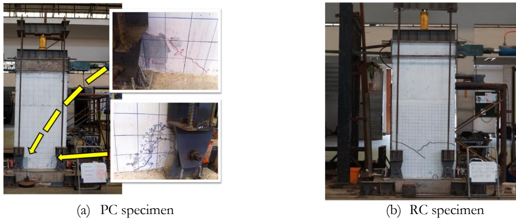
Fig. 14. Crack development in specimen.
