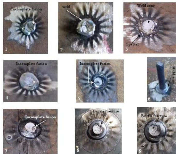
Fig. 9. The fractured specimens by torsional test.
