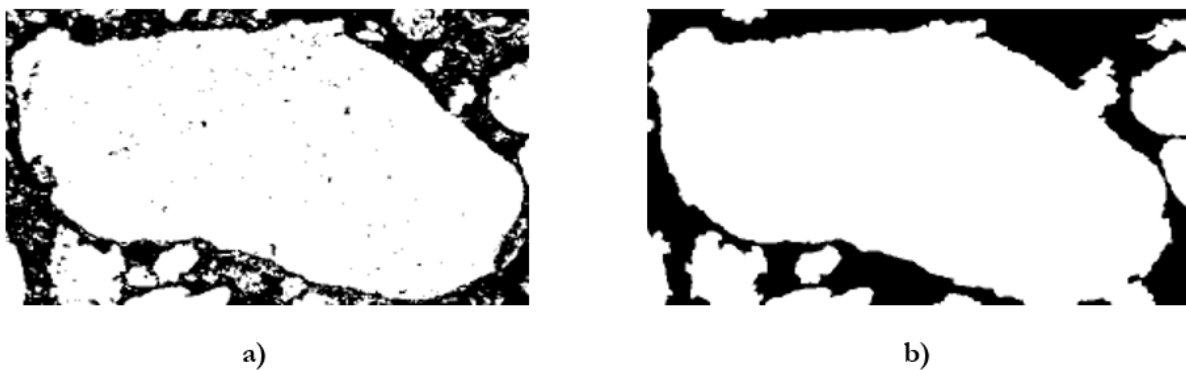
Fig. 4. Examples of the hole-filling technique. (a) Image with noise before and (b) after (the output) the hole-filling technique.
