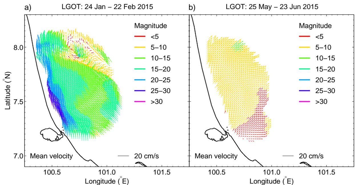
Fig. 5. Averaged surface currents over 720 hourly measurements at LGOT. Details are the same as Fig. 3.
