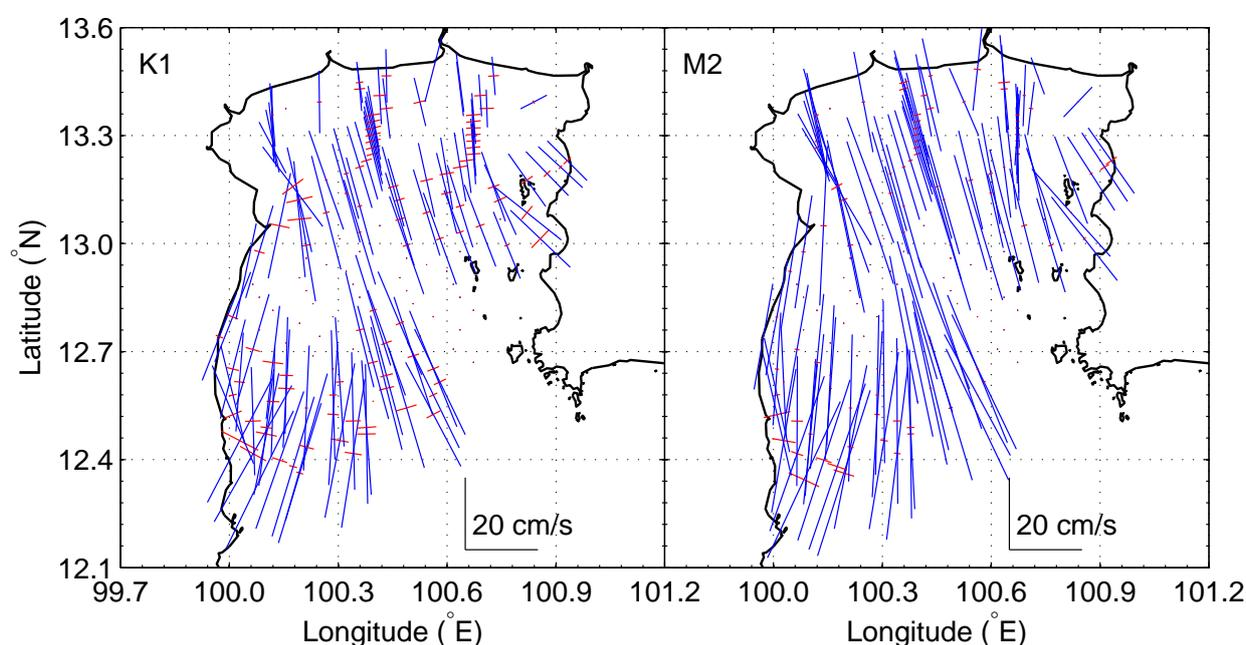
Fig. 7. Tidal ellipse parameters during the northeast monsoon at UGOT. Major axes (blue line) and minor axes (red line) of K1 (left panel) and M2 (right panel).
