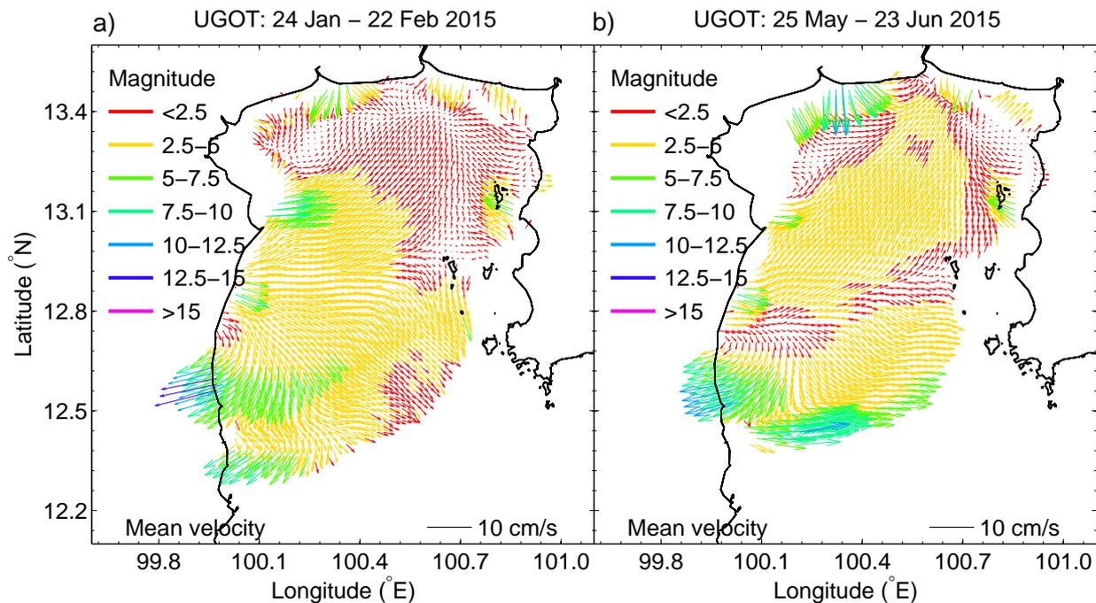
Fig. 3. Averaged surface currents over 720 hourly measurements at UGOT during two different monsoons: a) northeast monsoon (24 January - 22 February 2016); and b) southwest monsoon (25 May - 23 June 2016). Scale of the current is shown at the bottom.
