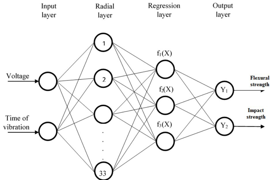
Fig. 8. GRNN architecture used for estimating mechanical properties.
