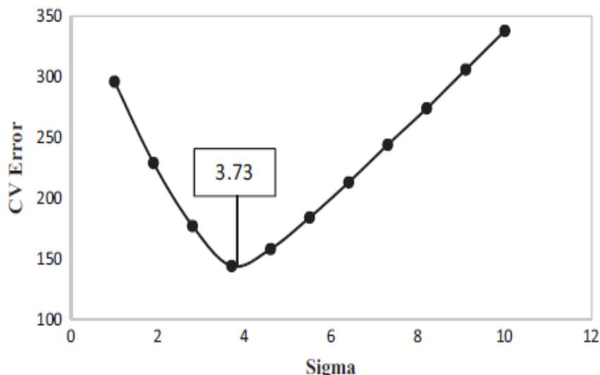
Fig. 9. Cross-validation graph for finding optimal kernel width.
