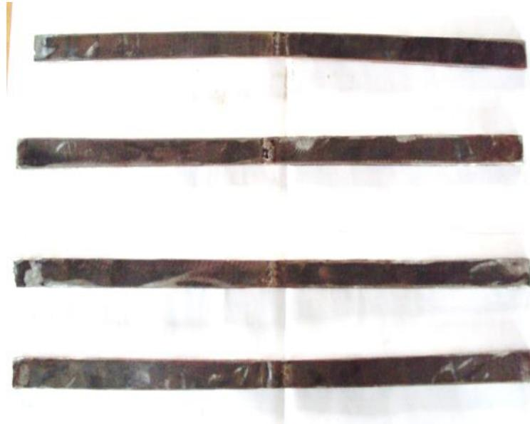
Fig. 3. (a) Produced specimens for Flexural test.
