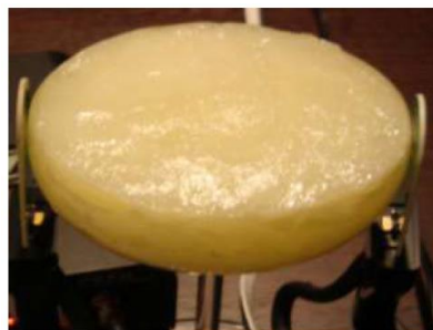
Fig. 10. Homogeneous breast phantom developed in [38]. Image is adapted from [38].
