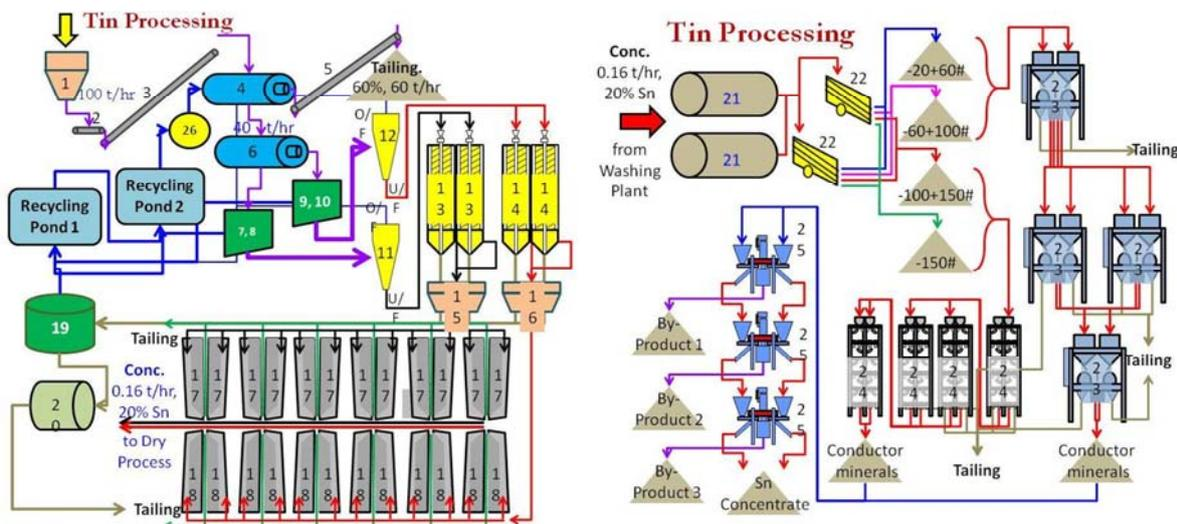
Fig. 9. Wet and dry dressing of the tailing dump.
