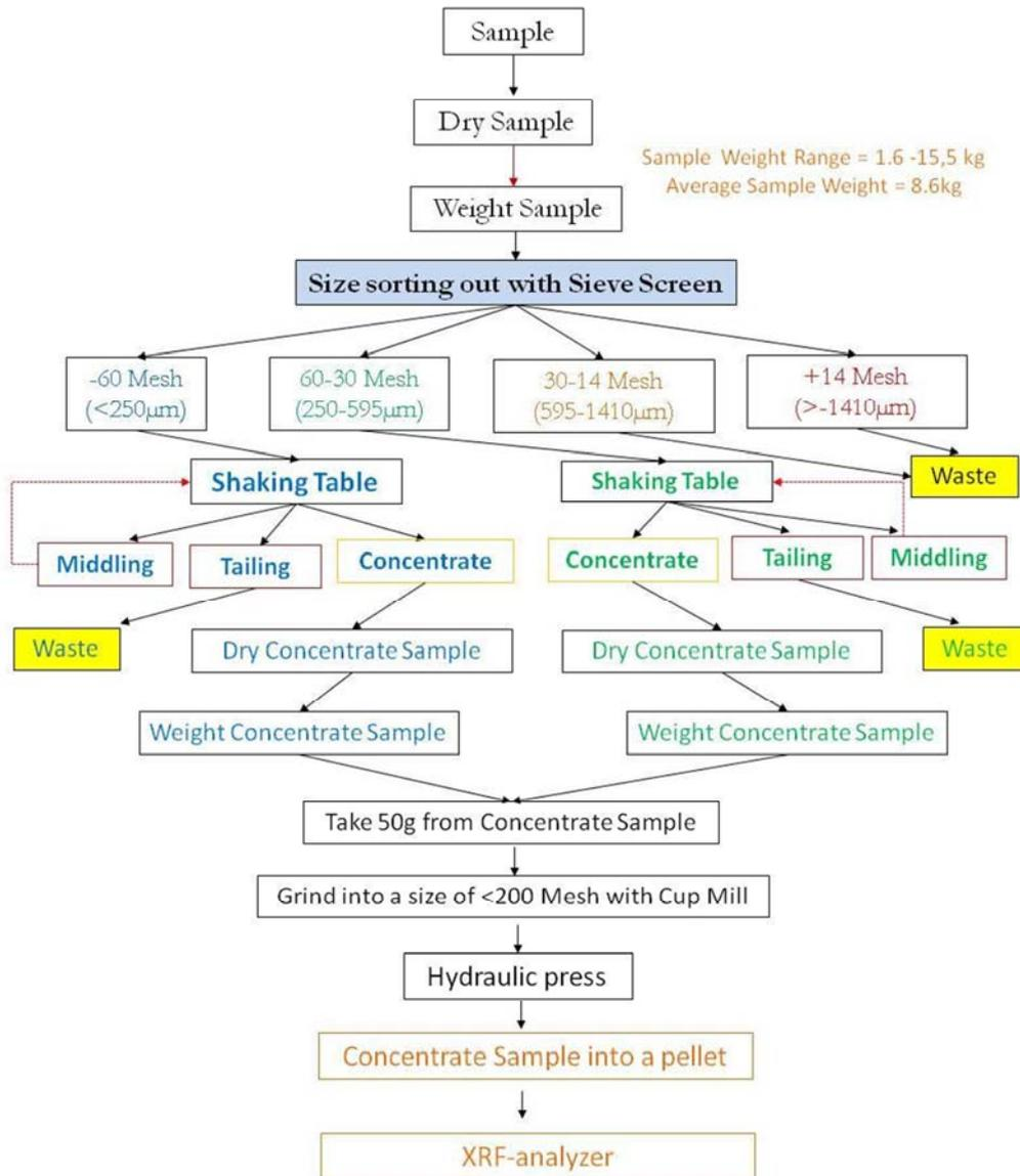
Fig. 8. Flow sheet of the chemical analysis and distribution of some valuable elements in the Jig tailings.
