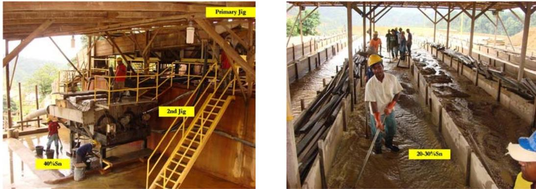
Fig. 2. Appearance of Palong, Primary Jig and Secondary Jig.
