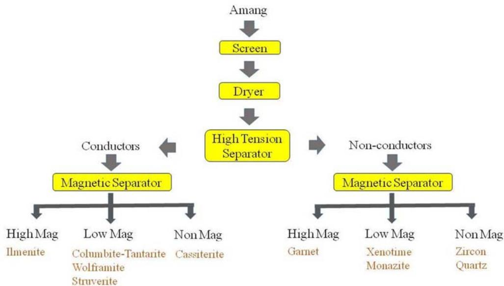
Fig. 5. Typical flow sheet of mineral processing from Amang.
