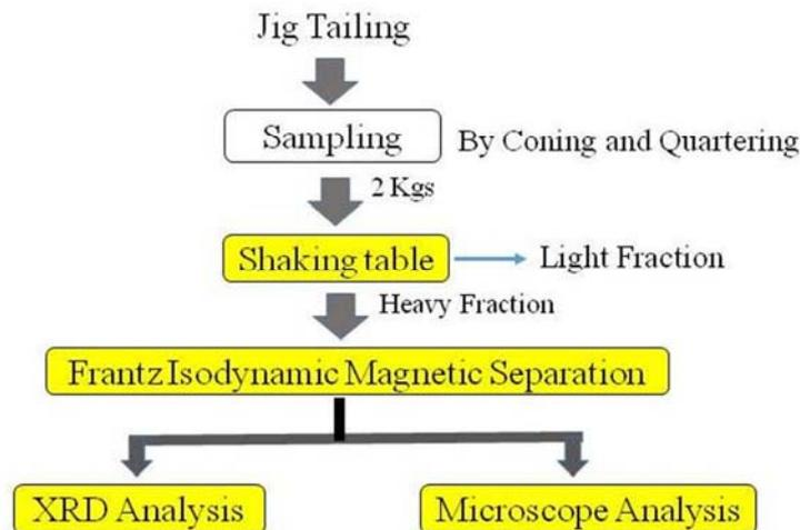
Fig. 7. Flow sheet of mineralogical study of Jig tailings.
