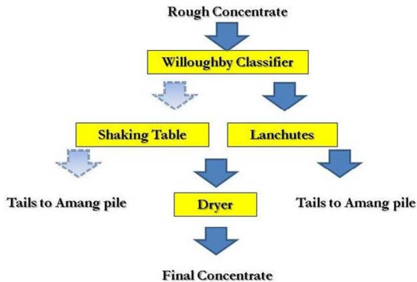
Fig. 3. Simple Dressing of Alluvial Tin Ore.
