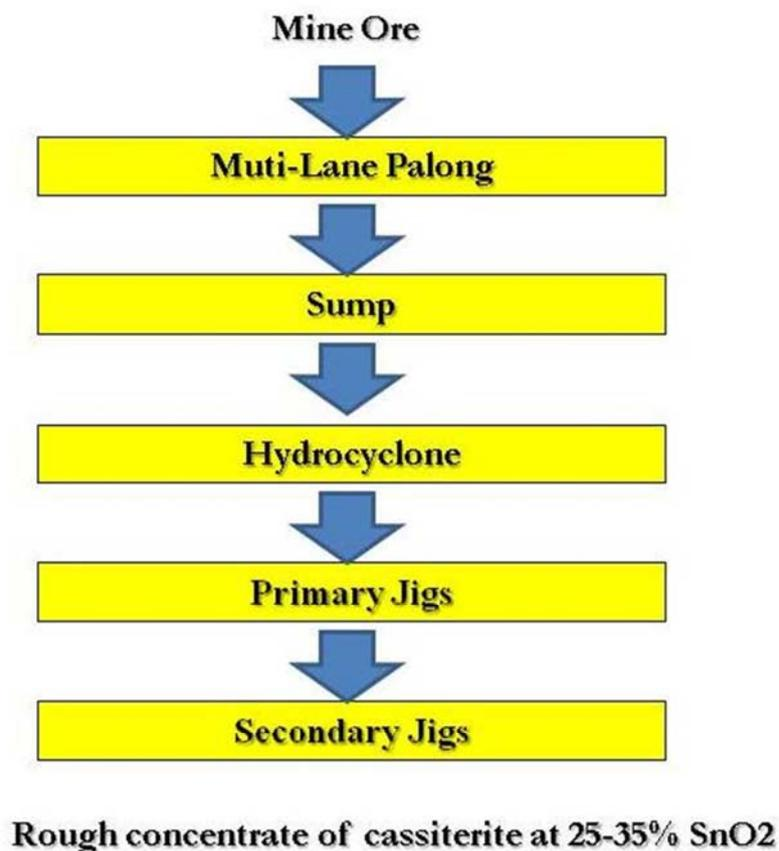
Fig. 1. Treatment of Tin Ore by Palong-Jigs system.
