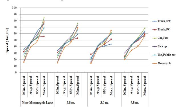
Fig. 4. Speeds of vehicle types in relation to varying MC lane widths.
