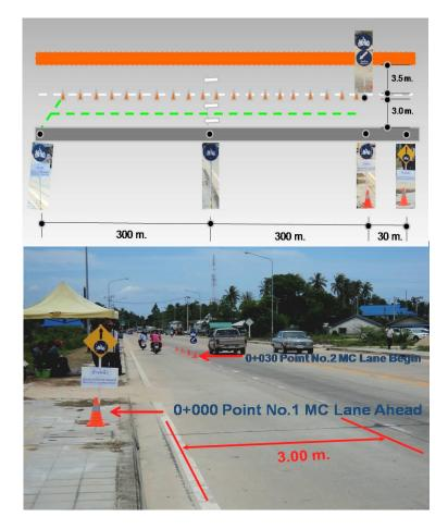
Fig. 3. Field test of MC lane configurations on an urban road in Narathiwas.
