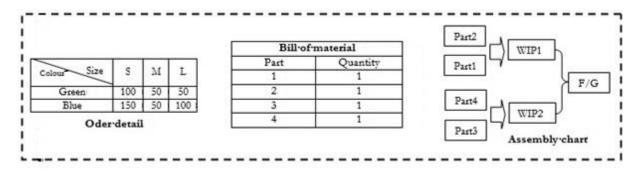
Fig. 6. Examples of order detail, bill of material, and assembly chart.
