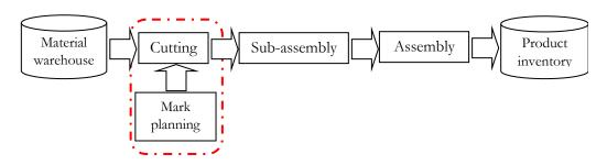
Fig. 2. The flow of garment processes with mark planning.
