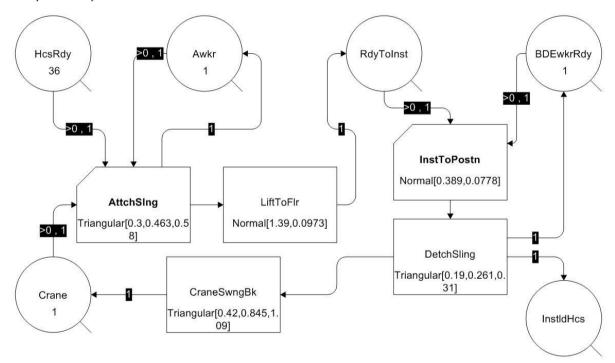
Fig. 3. EZStrobe ACDs showing installation works of 36 pieces of hollow-core slab.
