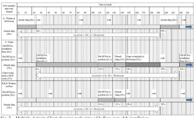
Fig. 2. Multiple-Activity-Chart showing cycle time of hollow-core slab installation.
