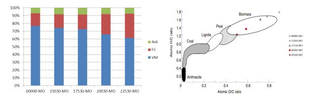
Fig. 11. Physical properties (left) and chemical properties (right) of raw and products from mixed organic waste.
