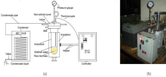
Fig. 1. Schematic (a) and installation (b) of lab scale reactor.
