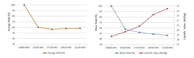
Fig 12. Effect of temperature on energy yield of mixed organic waste (left) and comparison between mass yield and calorific value of raw and products from mixed organic waste (right).
