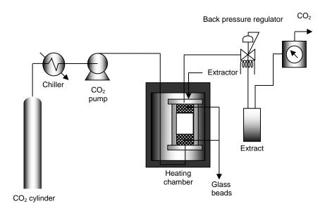
Fig. 1. Typical supercritical CO<sub>2</sub> extraction apparatus in laboratory–scale.
