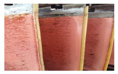
Fig. 13. Physical aspect of cathodic copper when solid colloidal particles and silica are present in aqueous solution at copper solvent extraction
