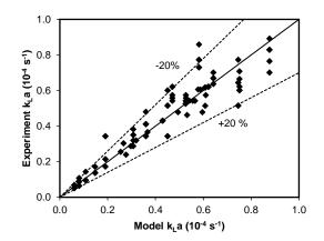
Fig. 8. Comparison of  $k_{La}$  from the experiment and the empirical correlation for aeration in hollow fiber membrane.
