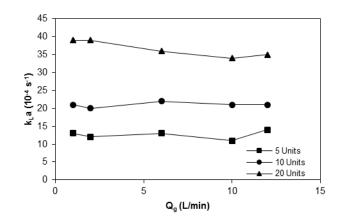
Fig. 6. Effect of number of hollow fiber membrane on the overall mass transfer coefficient ( $k_La$ ) in aeration system ( $Q_L = 0.1 \text{ l/min}$ ).
