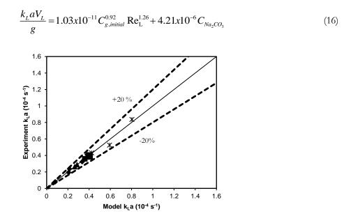
Fig. 11. Comparison of  $k_La$  from the experiment and the empirical correlation for CO<sub>2</sub> absorption in hollow fiber membrane.
