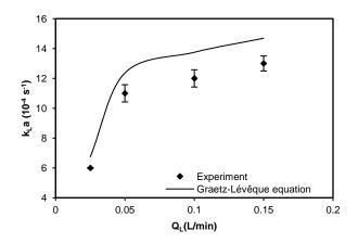
Fig. 5. Effect of the liquid flow rate on the overall mass transfer coefficient ( $k_La$ ) in aeration system ( $Q_g = 2 l/min$ , Number of membrane module = 5).
