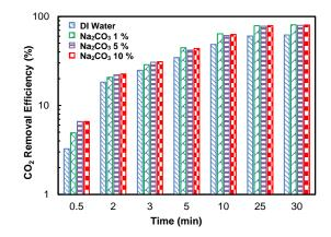
Fig. 10. Comparison of CO<sub>2</sub> removal efficiency between physical and chemical absorption.
