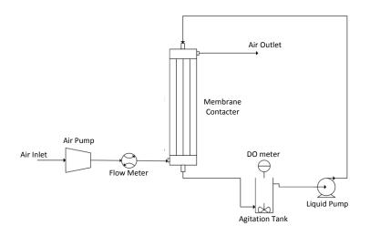
Fig. 2. Experimental set-up for aeration system.
