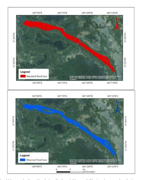
Fig. 3. Flood Map results from Simulation (Red) and Observed (Blue) at the same date (in Aguast 24, 2008).
