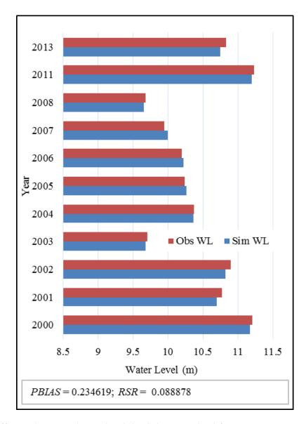
Fig.4. The difference between observed and simulation water level from 2000 to 2013 except 2009, 2010 and 2012.
