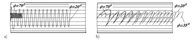
Fig. 6. Relative trajectories of particle sliding over an inclined cylinder ( $\beta$ =2<sup>0</sup>) at various combinations of angles  $\varphi$  and  $\psi$ : (a)  $\varphi$ =90<sup>0</sup>, t=10 s; (b)  $\varphi$ =45<sup>0</sup>, t=7 s.
