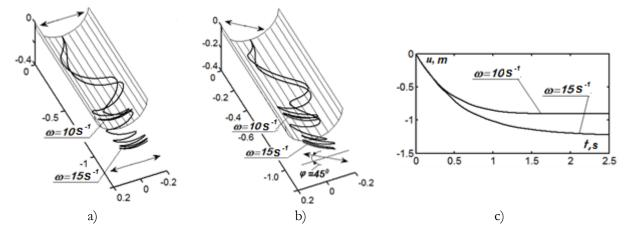
Fig. 3. Graphic illustrations of particle motion over a horizontal cylider, which performs rectilinear recipricating oscillations in a horizontal plane at initial velocity u'=2 m/s along its axis: (a) Trajectory of a particle at  $\varphi = 90^{\circ}$ ;
