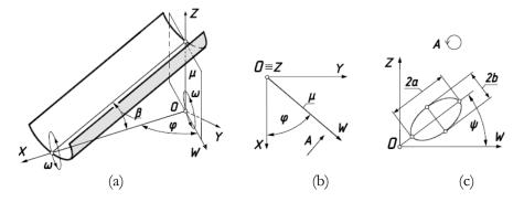
Fig. 1. Graphic illustrations of an inclined cylinder location and the direction of its oscillations: (a) Location of a cylinder in *OXYZ* coordinates;
