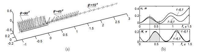
Fig. 7. Graphic illustrations of particle motion over a cylinder that is inclined at an angle  $\beta=2^{\circ}$ , the points of which trace circles:
