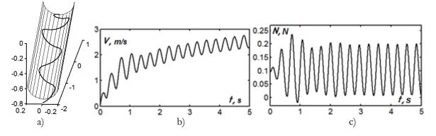
Fig. 5. Graphic illustrations of particle motion over a cylinder, which is inclined at a friction angle  $(\beta = \arctan \beta)$ , that performs reciprocating oscillations:
