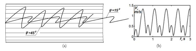
Fig. 8. Graphic illustrations of particle motion over a cylinder, the points of which move around a circle with angular velocity  $\omega = -10 s^{-1}$  and which is inclined at an angle  $\beta = 2^{0}$ :
