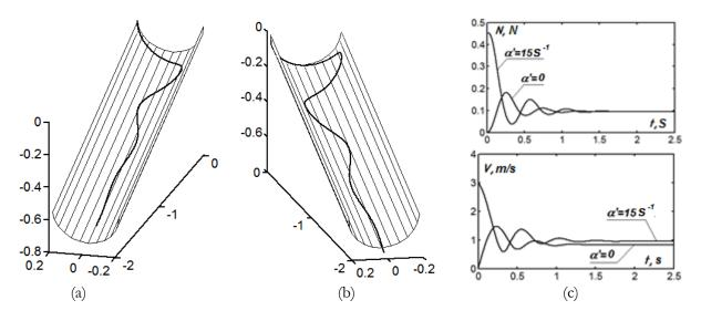
Fig. 2. Graphic illustrations of particle motion over a fixed cylinder, which is inclined at a friction angle  $(\beta = \arctan \beta)$ :
