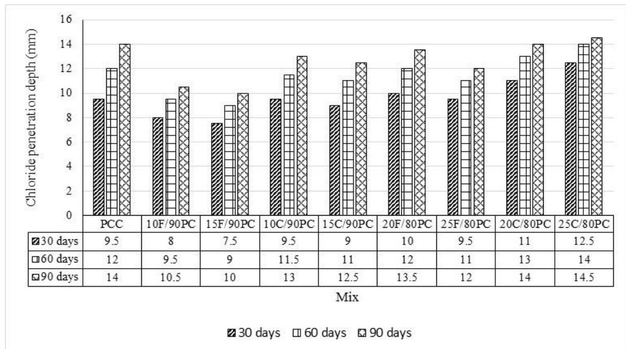
Fig. 2. Chloride penetration depth of full immersion in 3% NaCl solution.
