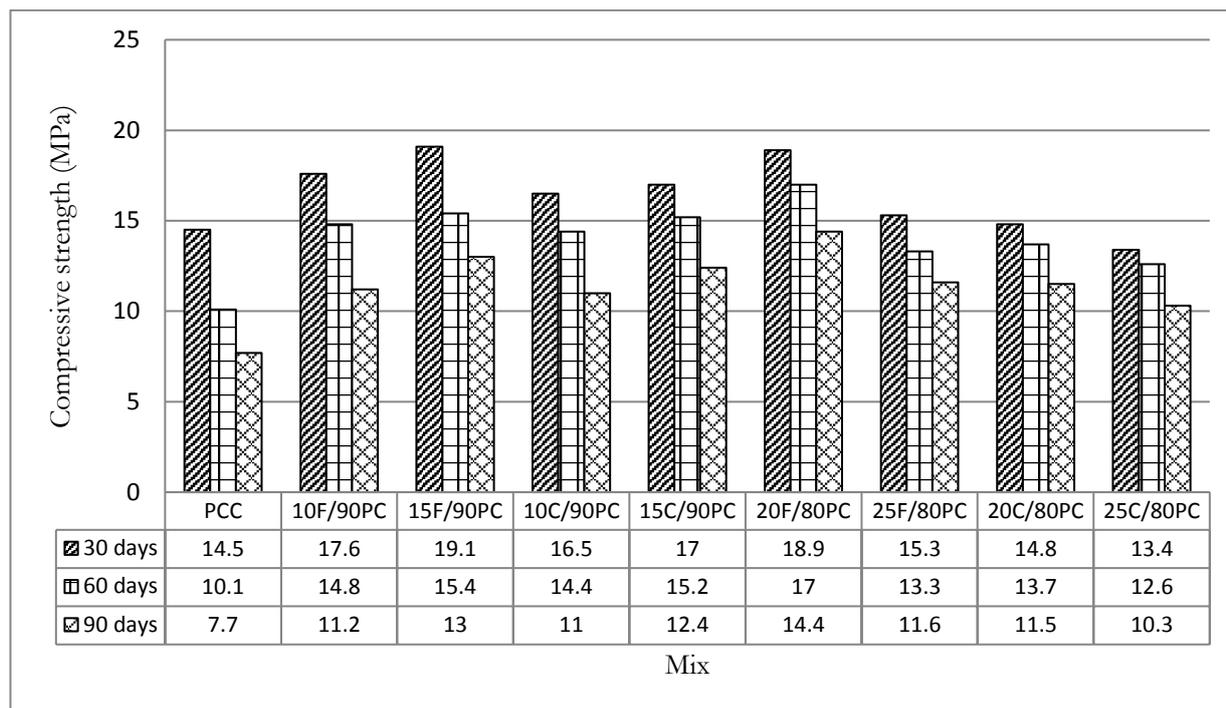
Fig. 4. Compressive strength of cube samples in 5% sulphuric acid.
