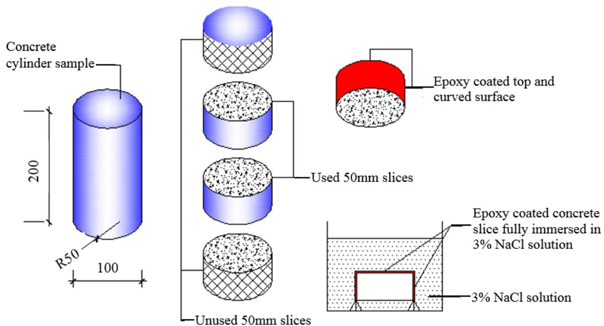
Fig. 1. Full immersion of concrete specimen in 3% NaCl solution [2].
