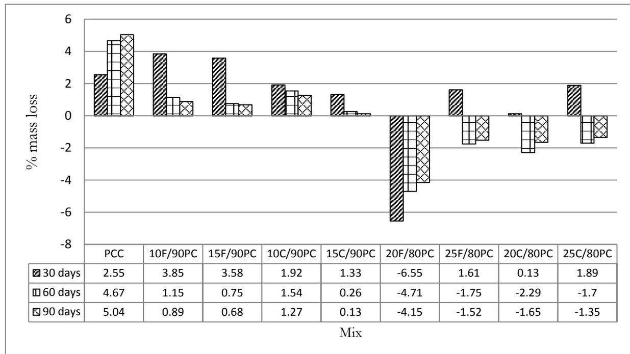
Fig. 6. Percentage mass loss of cube samples in sulphuric acid.
