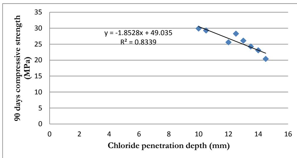
Fig. 3. Chloride penetration depth vs compressive strength at 90 days.
