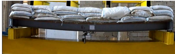
Fig. 17. Failure of control composite SB-RC deck floor (T SB-RC R ).
