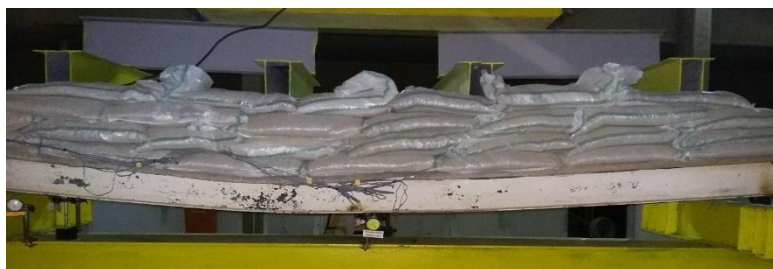
Fig. 19. Failure of burned composite SB-RC deck floor (T SB-RC500) after loading stage.
