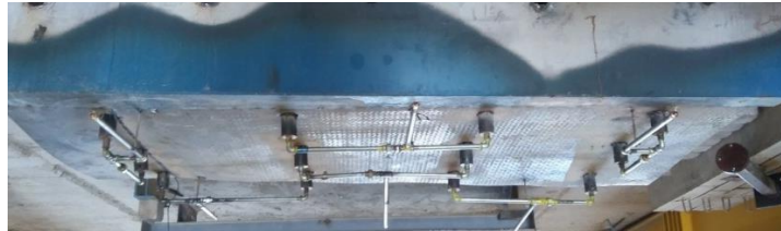
Fig. 3. Twelve nozzles to distribute fire flame underneath the specimen.
