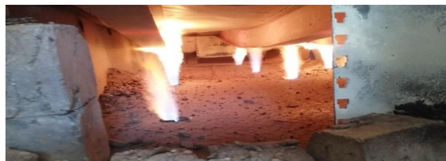
Fig. 4. Burning of specimen stage (Exposing to fire flam).
