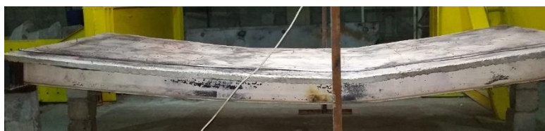
Fig. 20. Failure of burned composite SB-RC deck floor (T SB-RC700) after loading stage.
