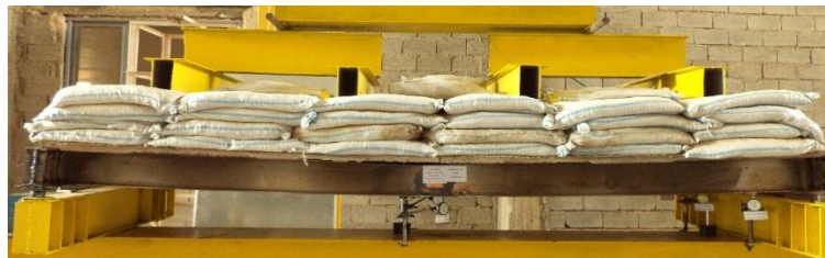
Fig. 18. Failure of burned composite SB-RC deck floor (T SB-RC300) after loading stage.
