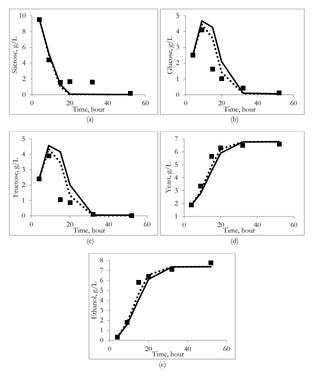
Fig. 5. Experimental data fitting using two proposed kinetics models of FS501 juice fermentation for: (a) Sucrose (b) Glucose (c) Fructose (d) Yeast (e) Ethanol (■: experimental data; —: Philippidis; ●●●: Philippidis – Modified).
