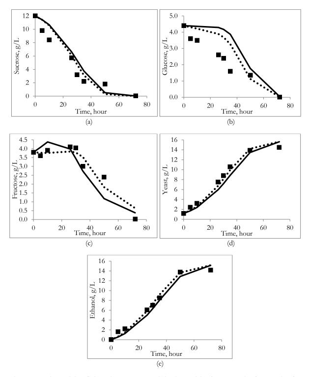
Fig. 4. Experimental data fitting using two proposed kinetics models of KCS105 juice fermentation for: (a) Sucrose (b) Glucose (c) Fructose (d) Yeast (e) Ethanol (■: experimental data; —: Philippidis; ●●●: Philippidis – Modified).
