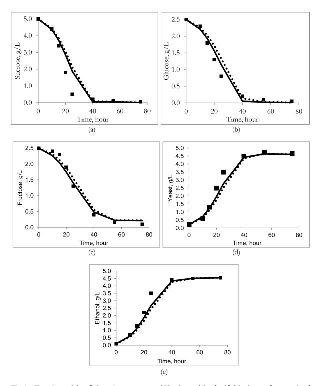
Fig. 3. Experimental data fitting using two proposed kinetics models of artificial substrate fermentation for: (a) Sucrose (b) Glucose (c) Fructose (d) Yeast (e) Ethanol (■: experimental data; —: Philippidis; ●●•: Philippidis – Modified).
