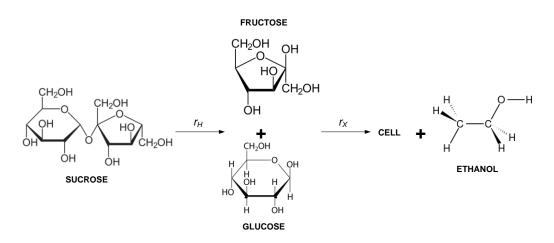
Fig. 1. Pathway of simultaneous hydrolysis and fermentation of sweet sorghum juice.
