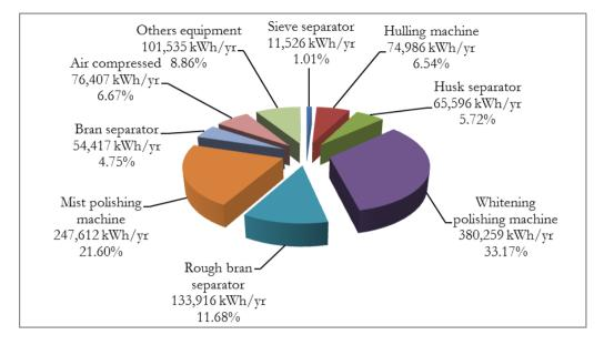
Fig. 2. The proportion of power consumption for each tooling process.
