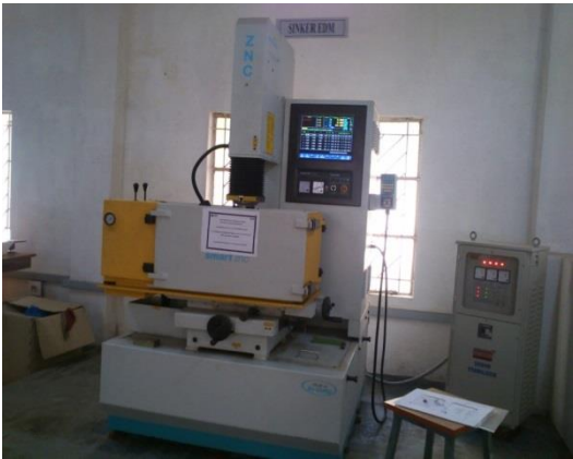
b. Electric discharge machine used for machining of Micro-grooves on the rake face of WC cutting tools
