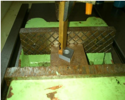
c. Setup of electrode and workpiece used for the experimentation
