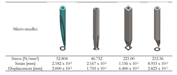
Table 9. Comparison of 20°, 40°, D1 and D5-2 tip micro-needle.
