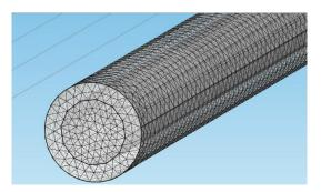
Fig. 4. Meshed model of dodecagon channel.
