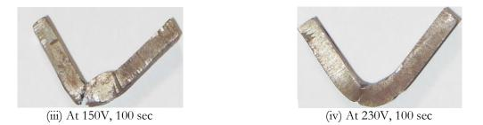
Fig. 5. (b) Specimens after impact failure.
