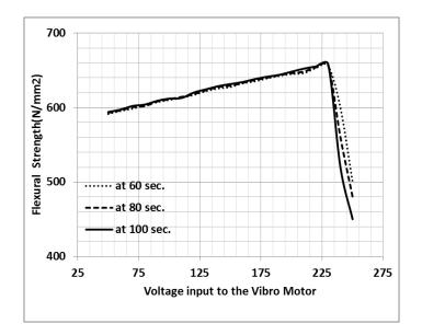
Fig. 4. Flexural strength variation with respect to input parameters.
