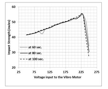
Fig. 6. Impact strength variation with respect to input parameters.
