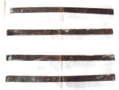
Fig. 3. (a) Produced specimens for Flexural test.
