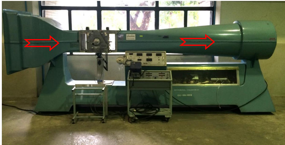
Fig. 4. The wind tunnel model WT300. Notice that, the arrow symbol is the flow direction.
