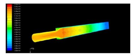
Fig. 3. Distribution of temperature for fuel element MTR use non porous media.
