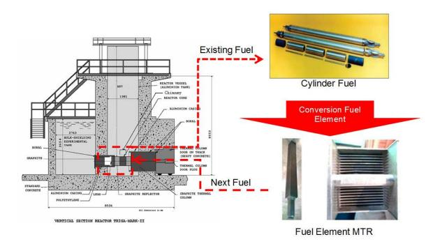
Fig. 1. Modification of Research Reactor TRIGA Bandung With Fuel Element Plat MTR.
