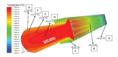
Fig. 5. Distribution of temperature for fuel element MTR [10].
