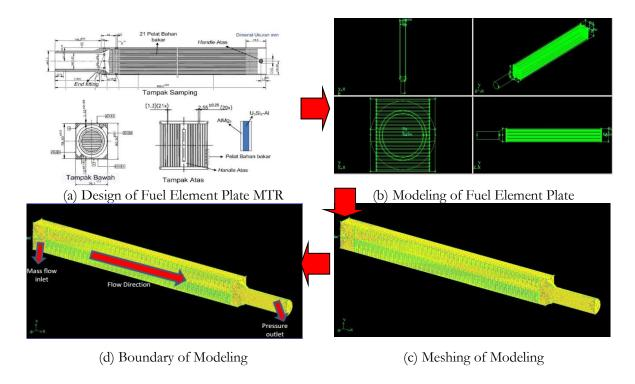
Fig. 2. Modeling of fuel element plate MTR.
