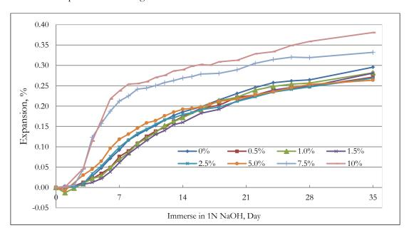
Fig. 6. Average expansion of mortar bars with synthetic zeolite and percentage replacement.
