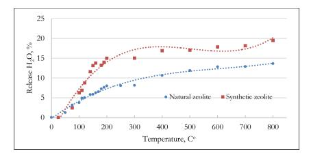
Fig. 3. Released water at different temperatures for both natural and synthetic zeolites.
