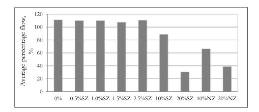
Fig. 4. Behavior on flow spread of mixtures.
