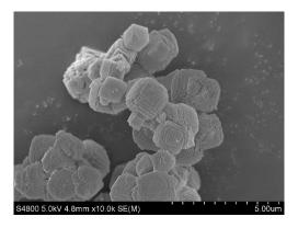
Fig. 1. Typical crystal shape of synthetic zeolite.
