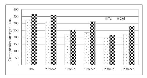
Fig. 5. Average compressive strength of mortar samples with different zeolite types and percentage replacement.
