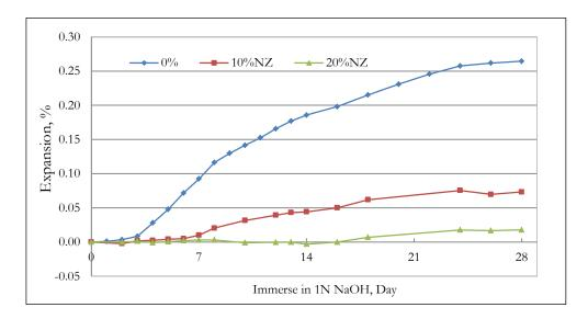
Fig. 7. Average expansion of mortar bars with natural zeolite.
